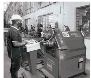
Profile Bending Machine
